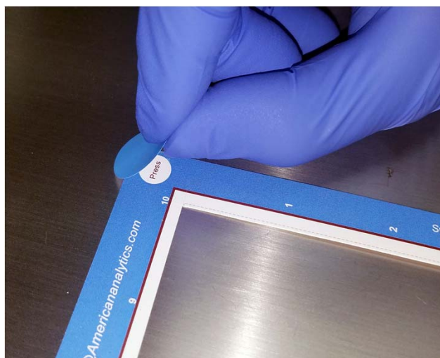
Figure: Applying the adhesive dots to position frame onto the intended wiping surface.
